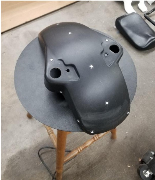
Figure 17. Fender and Infrared Targets
