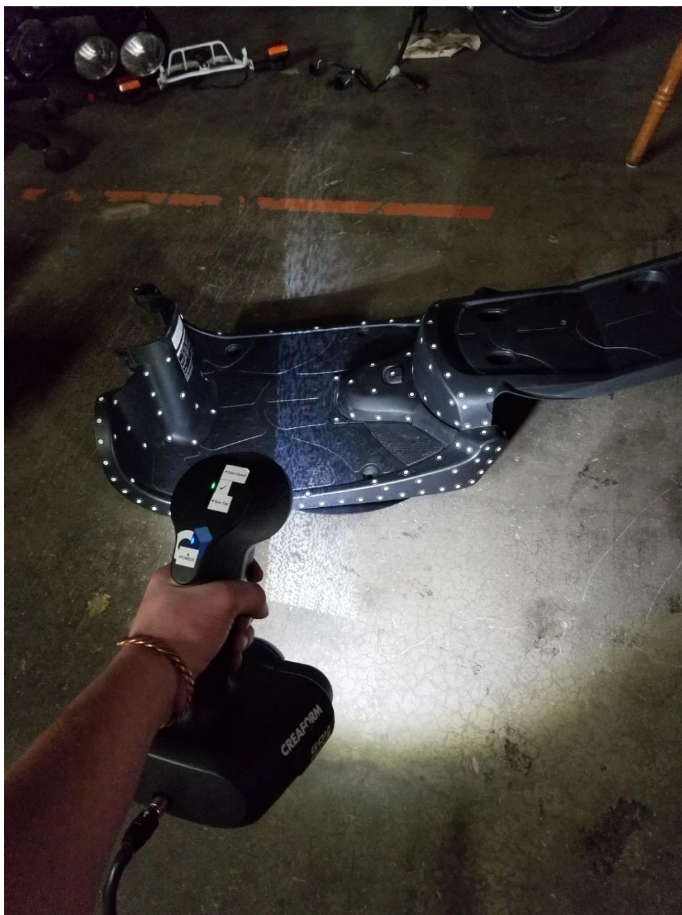
Figure 10. Scanner at the correct distance away from the floor panel.
