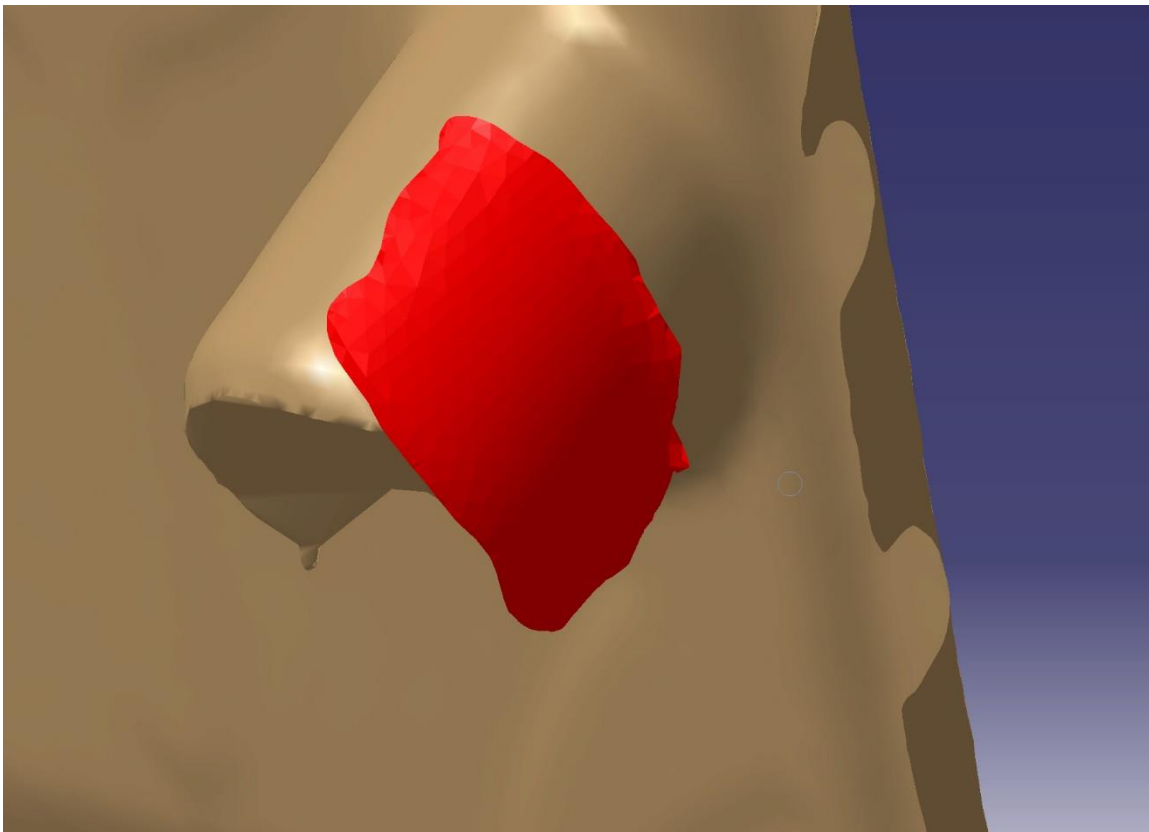
Figure 23. Example of added points that are not connected to the main mesh cloud and are able to be deleted without compromising the end product.
