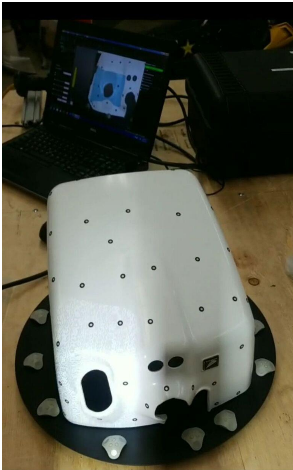
Figure 9. Battery housing with infrared positioning stickers and plastic positioning targets placed around it.
