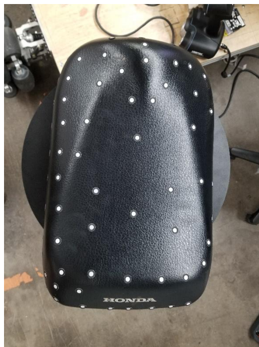
Figure 12. Infrared Targets Added
